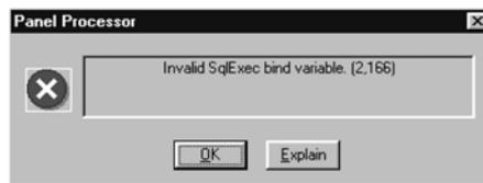
Figure 15.3 Runtime error using incorrect bind variable
